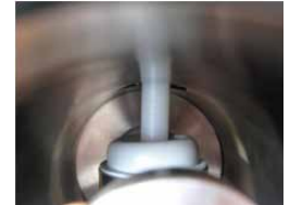
The beater is used for removing residues (when poor-flowing products are handled)
