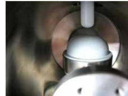
180° rotation of the cup; sample is tipped out in the down pipe
