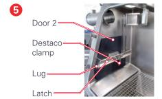
Reach into the gloves and open the Destaco clamps.
