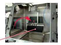
6 Use the gloves to pull the sack into the glovebox.
