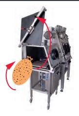
3 Lower door 1 using the black handle. Lock door 1 using the Destaco clamp.
