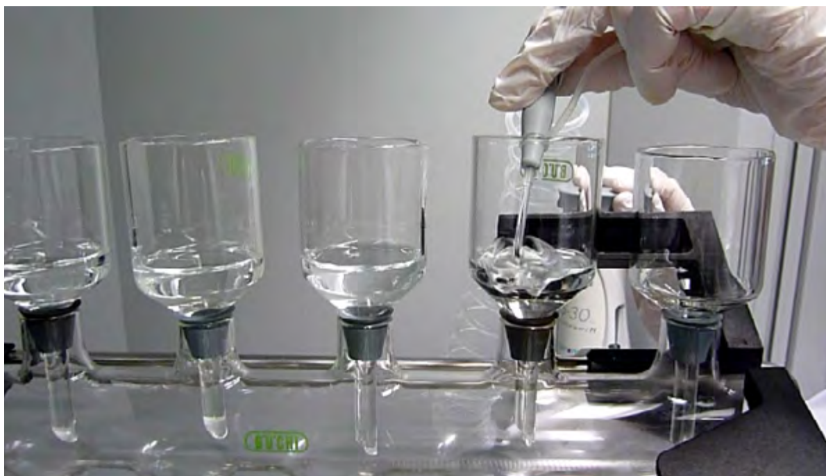
Addition of hydrogen peroxide into capillary funnels during digestion
