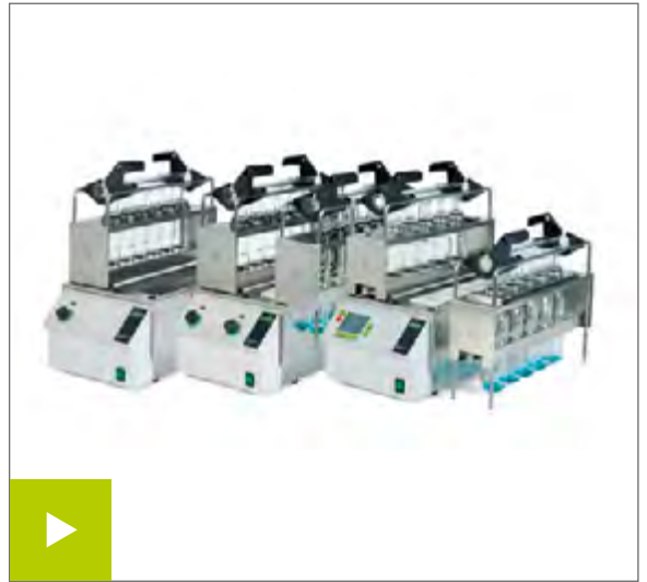
SpeedDigester K-425 / K-436 / K-439 with Kjeldahl setup
